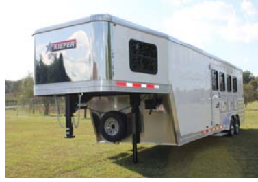
Stainless Nose/.050 Aluminum Exterior
